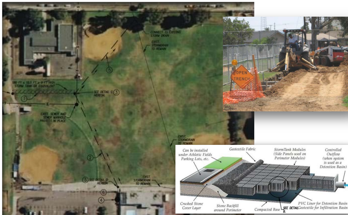
Figure 3-8 Schematics & Construction Photos for the Memorial Park Infiltration Basin
